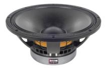
The B&C 15RBX100 anchors our ferrite subwoofer line, and features an all new FEA optimized motor structure. The 25mm high, 4" (100mm) diameter copper wire voice coil is combined with a laminated double silicone spider, water resistant curvilinear cone and triple roll surround, for even more excursion and linearity.
